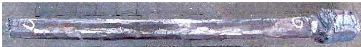
Fig. 1. Experimental shaft forged from the 100 kg ingot
